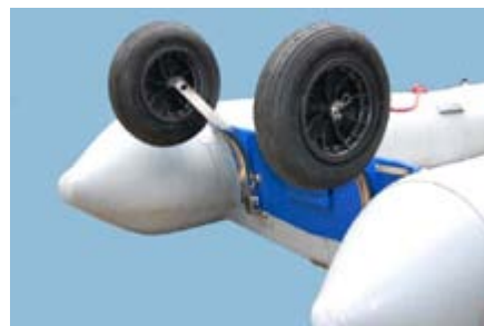
#1483 Wheel-a-Weigh Extra Duty with 14" (36 cm) inflatable tires and roller bearings inside hub. Curved wheel frames pivot under the boat for better balance.
